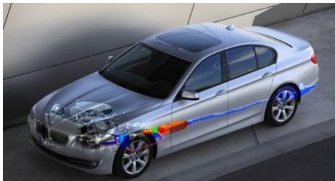
Recovery of thermal waste BMW TEG
