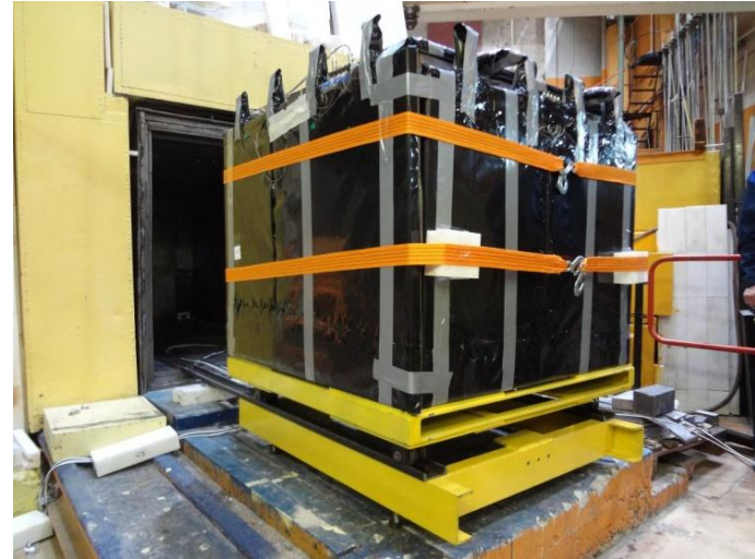
Detector with active shielding 4\pi
