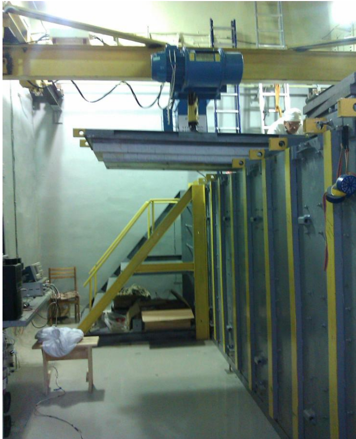
Passive shielding of 60 tons
