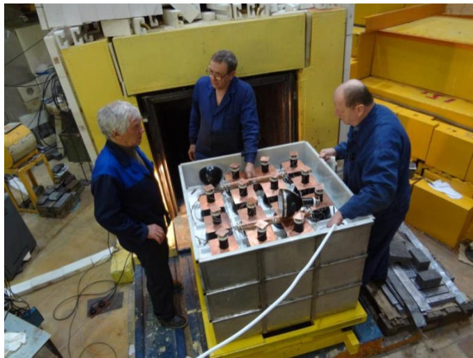
Filling by liquid scintillator 400 liters
