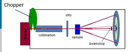
Simultaneous coverage of a wide Q-range, but lower intensity:
