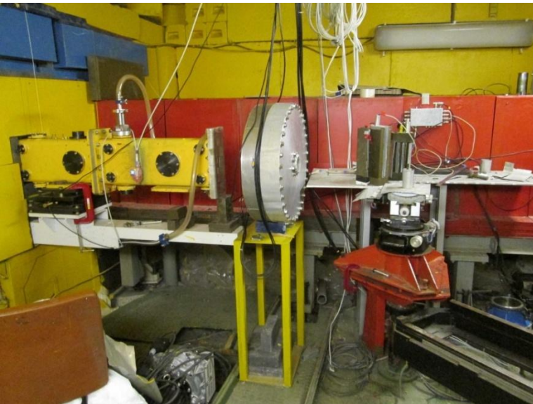
Ring-shaped helium backscattering detector on the RTD diffractometer
